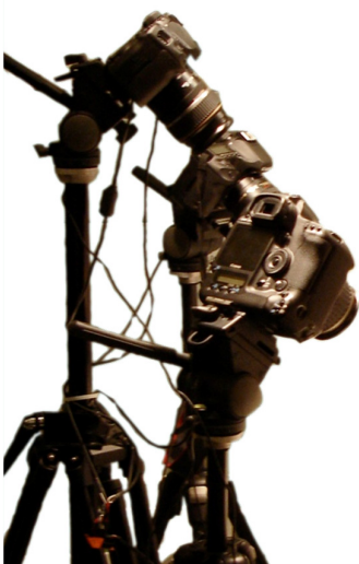
3 Canon 40D cameras External trigger for sync
