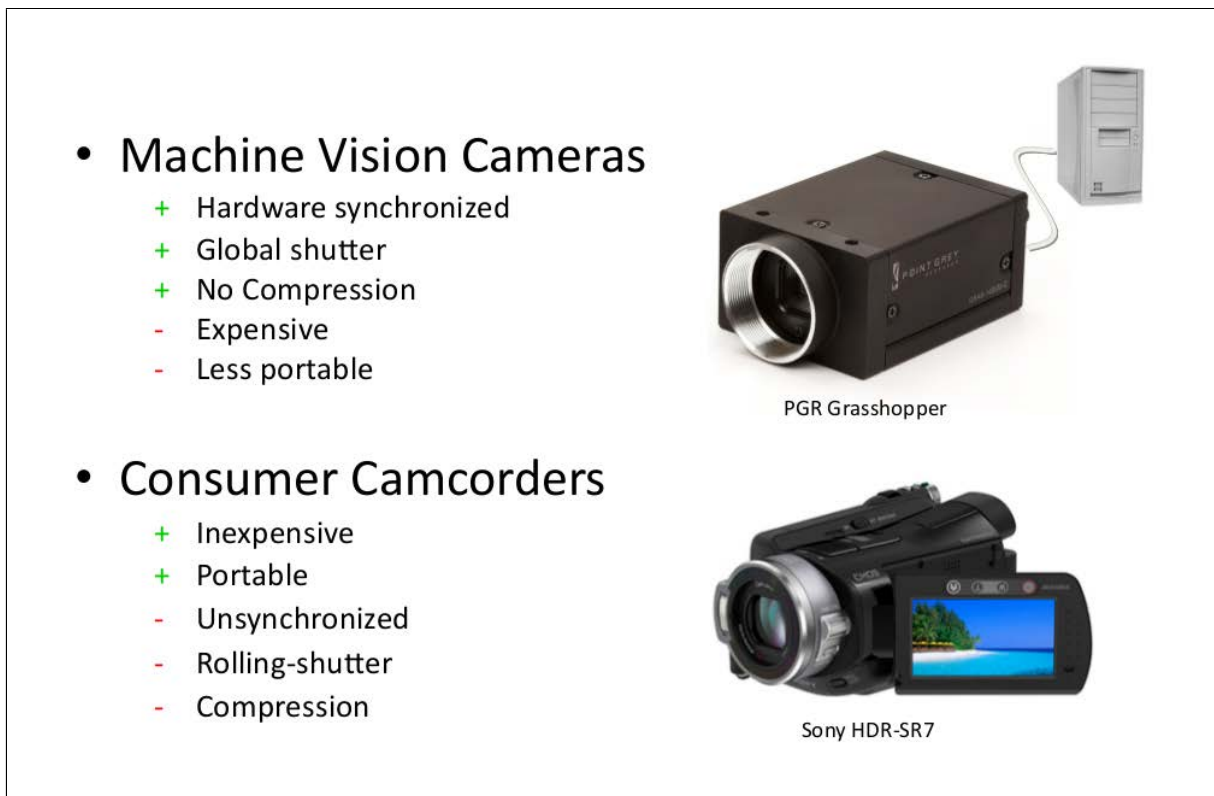
Figure 7: Trade-offs between machine vision cameras and consumer camcorders.
