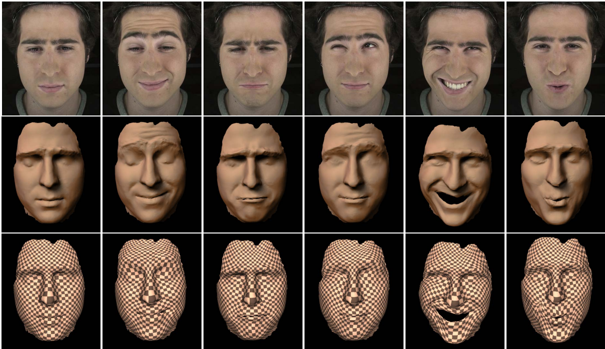
Figure 17: Deforming face reconstructions from Bradley et al. [2010]. The top row is a reference image, middle row shows the resulting geometry, and bottom row shows the reconstructed motion using an overlaid checkerboard pattern.
