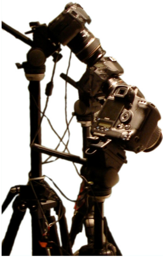
3 Canon 40D cameras External trigger for sync
