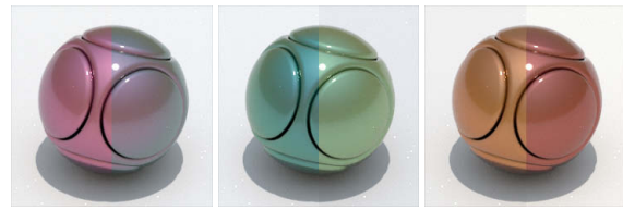
Figure 8: Spheres coated with three different effect lacquers of the type described by [SMAS08], without (left half of images) and with (right half) anomalous dispersion of the pigment particles taken into account. Apart from the dispersion characteristics of the pigments, the BRDF parameters (and in particular, the absorption characteristics of the pigment particles) are identical.
