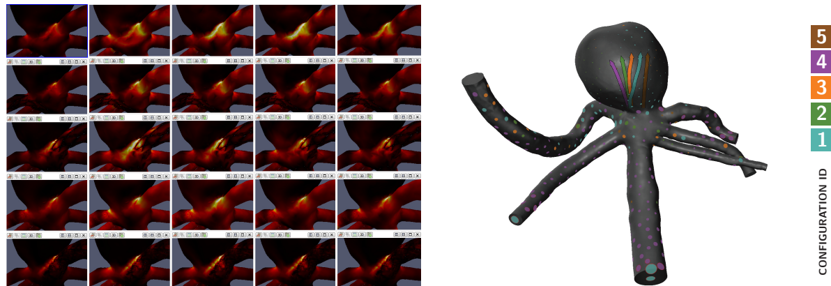
Figure 5: An informal evaluation was conducted with domain experts. They were presented with the established juxtaposed grid visualization (left) to compare the hemodynamic information of different stent configurations, and were asked to compare this to our comparative visualization approach (right). Besides the WSS values on the vessel wall, our approach furthermore superimposes endovascular blood flow information, e.g., the inflow jets (dataset 1).
