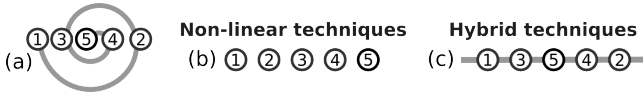
Figure 1: Dimensionality reduction with landmarks. In non-linear embedding techniques the underlying manifold (a) is respected (b). In hybrid approaches, landmarks are placed without considering the underlying manifold (c) and data points are placed by interpolating the landmark positions (grey line in c). The layout quality thus relates to the used number of landmarks.
