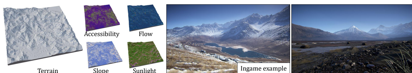
Figure 1: A typical example of terrain authored by artists for a AAA game: given an input low-resolution model composed by assembling major landforms, a high-resolution elevation model augmented with details is generated after computing the slope, sky illumination, accessibility, and drainage, not only to amplify the elevation but also synthesize vegetation occupancy and plausible village settlements.
