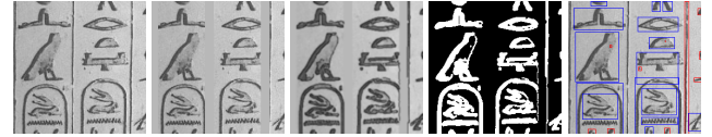
Figure 1: Generation of pseudo-labels. From left to right: Input image; Vertical lines removed; Edges enhanced; Otsu’s binarization; CCL applied; Blue boxes are kept as pseudo-labels, red ones are removed.
