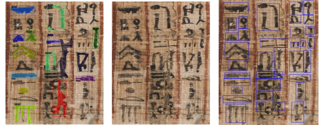
Figure 2: Detection on a difficult image taken from [GPF*23]. Left: Segmentation results from [GPF*23]; Middle: Input; Right: Our detection with the same model as in Figure 4. The model of [GPF*23] struggles to detect hieroglyphs and instead detects some artifacts, whereas our approach detects almost everything correctly.
