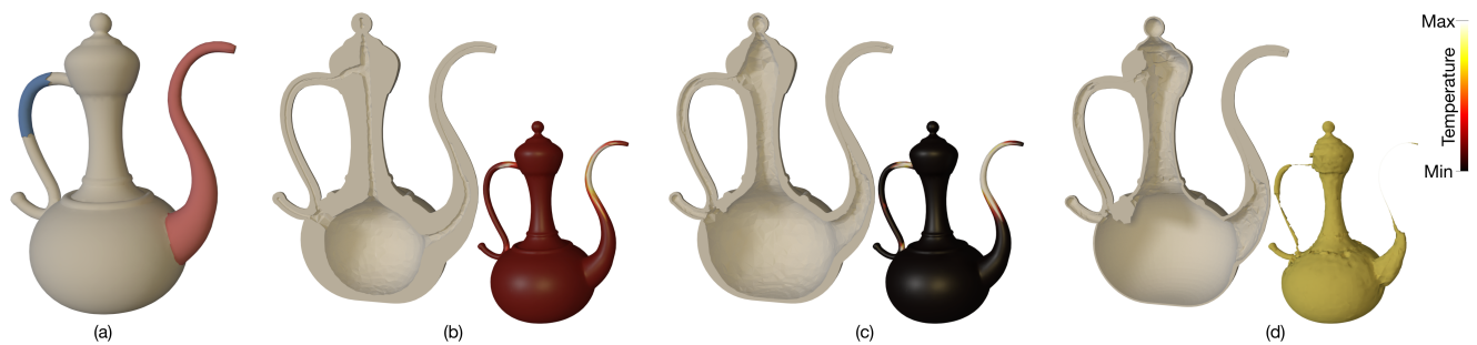
Figure 3: Given a contact region (red in a) where arbitrary forces can be applied on, our algorithm optimizes the boundary thickness locally (b-c) to find the smallest weight shell structure (d) that can withstand all possible force configurations. In (b-c), we show the material distribution in two steps of the optimization. Inset figures illustrate the scalar temperature fields on the boundary that we use to drive the shell thickness in (b-c) and the removed material in (d).
