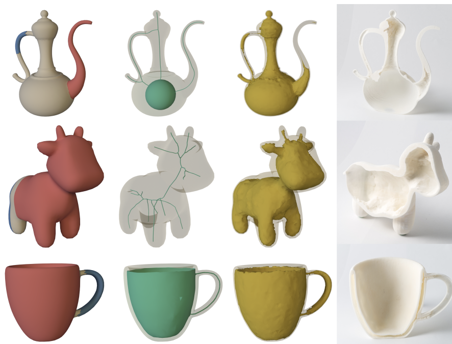
Figure 13: Structural optimization results for problems with force location uncertainties. Left-to-right, problem setups with fixed boundary conditions (blue) and force contact regions (red), skeletons used during the optimization, optimized shell structures and their 3D printed cut-outs revealing the variations in the shell thickness. Yellow surface indicates the inner boundary of the shell.
