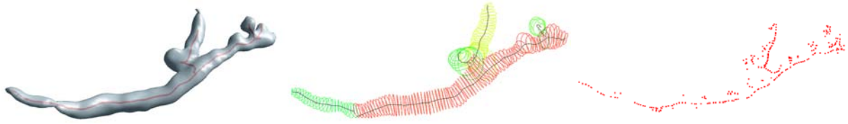
Figure 5: Our approach faithfully extracts a vortex core line that consists of several connected components (left). The approach by Stegmaier et al. extracts components of the vortex core line that are equivalent to our results but remain unconnected (middle). The \lambda_2 -based parallel-vectors approach extracts unconnected points on the vortex core line; several outliers are present as well as sections where no core line points were detected (right).
