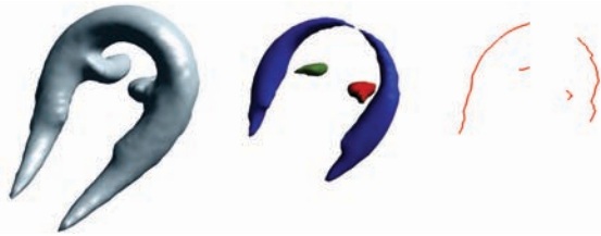
Figure 6: Semi-automatic isovalue determination: original vortical region (left); decomposition with color coding by isovalue (middle); the respective vortex core lines (right).
