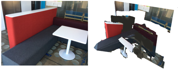
Figure 10: Failure Case: For this input scene (left) where there are many intersecting objects we are unable to accurately fit primitives and determine occlusions (right). Without accurate proxies we are unable to correctly complete the scene or synthesise new views.
