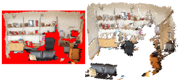
Figure 3: Example RGB-D input: Point cloud rendered from original camera pose (left) showing large regions of missing depth information labeled in red. When rendered from a different camera pose (right) the point cloud reveals many points have mislabeled depth values. The coarseness of the data emphasises the need for decomposing the scene into geometric proxies.
