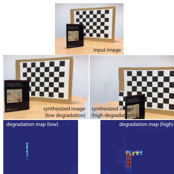
Figure 7: Novel View Synthesis: Input image (top) is used to create two novel views (middle) with degradation models (bottom). The left example has a low degradation score as the revealed region only has moderate texture and is close to known pixels. The right example has a high degradation score as it reveals a high texture region and far from known pixels.
