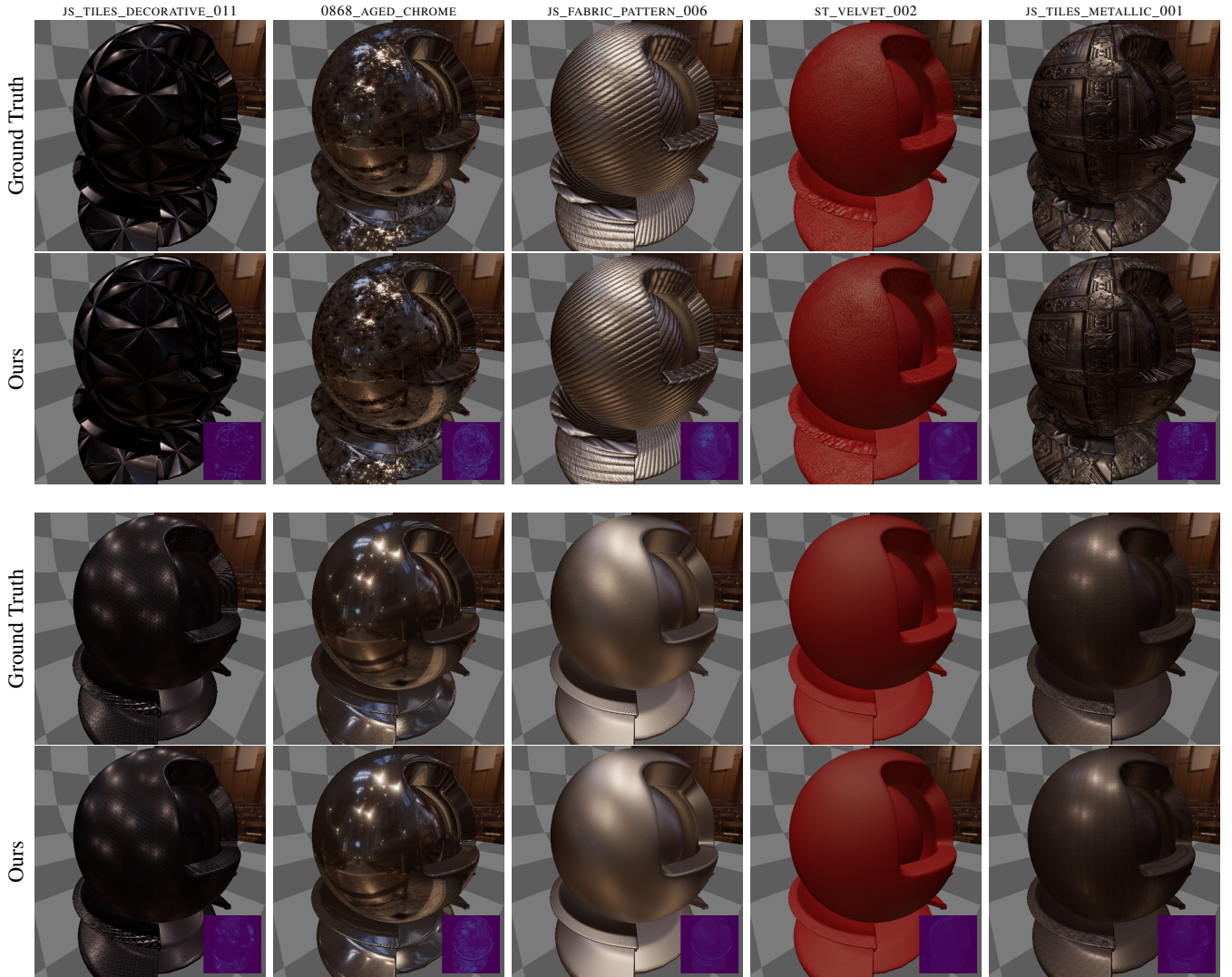
Figure A.10: Flexibility of our model trained demonstrated on MatSynth materials. We illuminate the object with the Grace cathedral [Deb98] environmental light with and visualize the object in two different scales (top and bottom groups). We use the importance sampler of the underlying ground truth GGX model. The errormaps visualize FLIP with respect to the ground truth.
