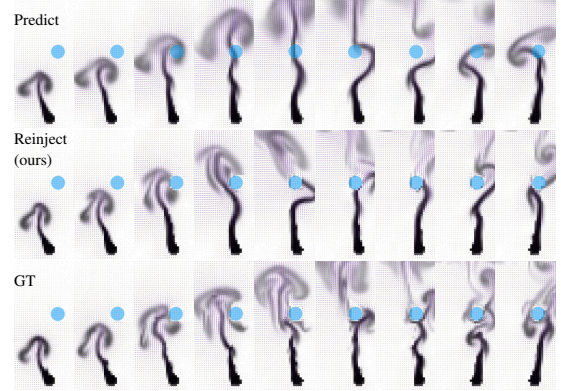
Figure 12: A circular solid obstacle, unseen during training, is placed in the upper right. The prediction of our proposed method (center) is stable and realistic. The prediction-only approach (top) is not able to capture the obstacle.
