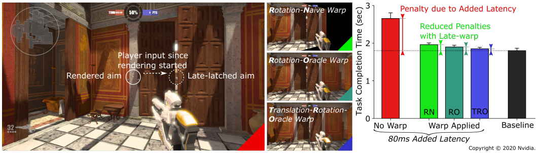
Fig. 1. Player view and key result from our experiment. Left : In traditional graphics pipelines, the generated image reflects the player input before rendering. Center : Late-warp updates the image based on late-latched player input. Right : Average task completion time shows a significant player performance penalty between 105 ms (No Warp) and 25 ms (Baseline) latency conditions. Error bars indicate the standard error of the mean of individual median scores (see Section 4). All warp methods tested mitigate this penalty.
