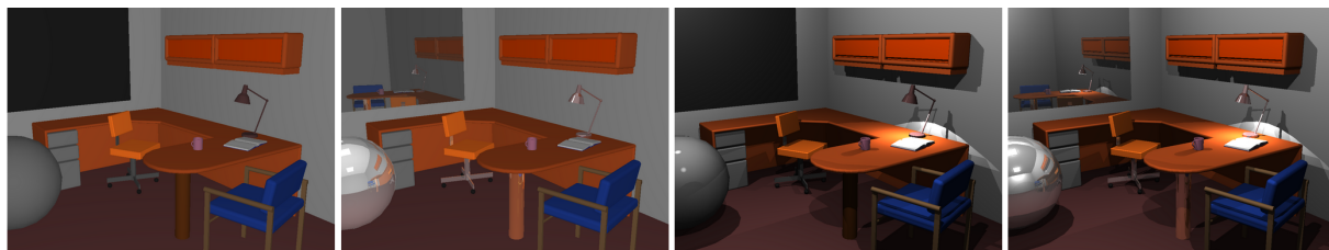
Figure 7: The Office scene with (from left to right): eye rays only ( er ); er and reflections; er and three point lights; er , reflections, and three point lights. It shows that the performance scales linear in the number of rays shot and independent of the type of the ray, i.e. eye, reflection and shadow rays have roughly the same cost. See Tables 5 and 6 for details.
