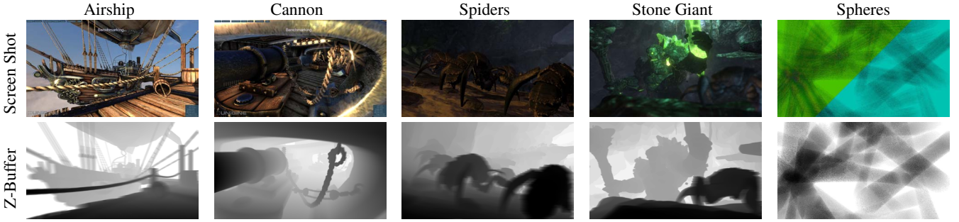
Figure 5: Images from the test scenes used to generate our results. The images are taken from the Heaven benchmark and Stone Giant demo and feature highly tessellated geometry. The Spheres scene is a synthetic benchmark scene intended to stress test highly varying motion. The top row contains reference screenshots without motion (except for the Spheres scene which includes motion), and the bottom row shows depth buffers, rendered using our rasterization framework, including motion blur. All images were rendered at 1920 \times 1080 pixels resolution. The images Airship and Cannon images are courtesy of Unigine Corp., and the Spiders and Stone Giant images are courtesy of BitSquid.
