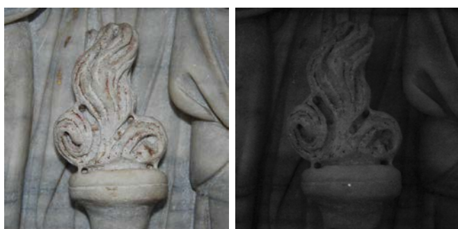
Fig. 10. Thymiaterion flame polychrome detail (left) and the same area in VIL imaging that shows the distribution of glowing white particles of Egyptian blue (right). On the flame the EB is located as scattered particles, while on the shaft shows a enough compact layer.
