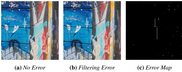
Figure 6: Comparison of filtering artifacts. (a) The clean reference image. (b) The image exhibiting artifacts due to missing MCUs for filtering. (c) An error map highlighting the pixel differences in white.
