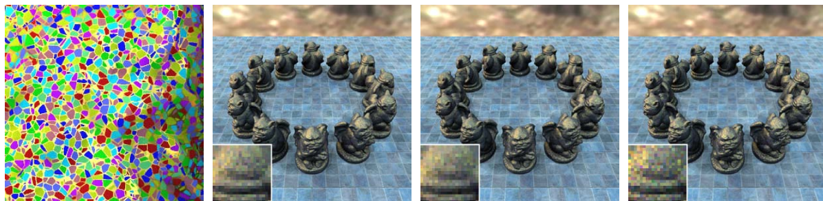
Figure 7: Cloisonné gargoyles. From left to right: a close-up view of the micro structures of one gargoyle, a ground truth rendering, a rendering using CPMs and an equal time budget rendering of the original model.
