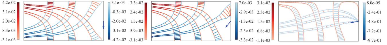
**Figure 6:** Coherence of conforming lattices that are generated automatically from the leftmost lattice when different load conditions (indicated by blue arrows) are applied to the 2D cantilever (Fig. 7a).
