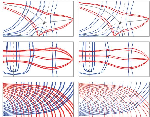
**Figure 8:** Top to bottom: Support trajectories for the 2D cantilever under different loads before (left) and after (right) optimization, including degenerate points (small circles), and the topological skeleton with PSLs along the major (grey solid lines) and minor (dashed lines) principal directions.
