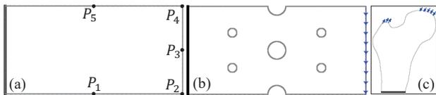
**Figure 7:** The 2D solid objects used in our experiments. Blue arrows indicate the load conditions. (a) Cantilever with fixed left edge, discretized into  $250 \times 500$  finite elements. Points  $P_1, \dots, P_5$  indicate the positions where different loads are applied. (b) Perforated plate, adapted from the cantilever. (c) Slice through a 3D CT-scan of a femur; fixed at the bottom and discretized into  $182 \times 140$  finite elements.
