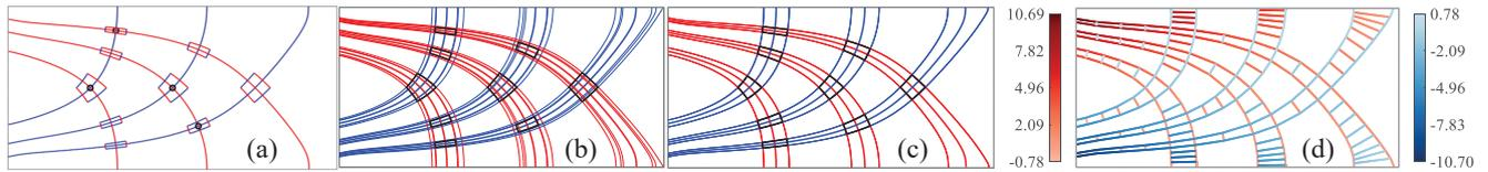
**Figure 3:** Method overview: (a) Selected nodes (black circles) and computed intersections, skeleton trajectories, seed elements oriented along PSLs. (b) Edges of connected nodes do not lay on the same PSL, (c) but do so due to anisotropic scaling during optimization. (d) Conforming lattice, where beams of elements connect the seed elements. Coloring indicates stress magnitude, tension and compression.
