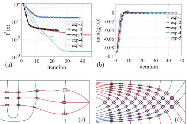
**Figure 12:** Top: Convergence analysis for all 2D experiments. (a) Normalized objective function. (b) Constraint function. Bottom: Comparisons of seed elements before and after optimization, for the 2nd (c) and 3rd (d) test case. Elements with colored edges depict the initial seed elements, black edges indicate optimized elements.
