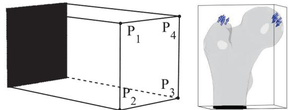
**Figure 14:** The 3D solid objects used in our experiments. Blue arrows indicate the load conditions, regions where the objects are fixed are shown in black. Left: 3D cantilever with fixed left face, discretized into  $50 \times 100 \times 50$  finite elements. Different loads are applied at points  $P_1, \dots, P_4$ . Right: Femur fixed at the bottom, discretized into  $140 \times 92 \times 182$  finite elements.
