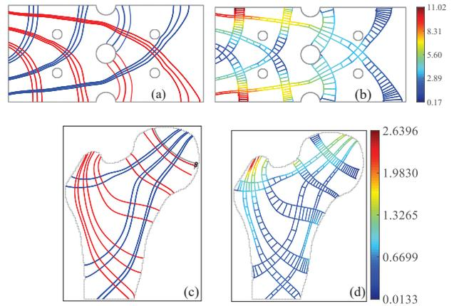
**Figure 11:** Perforated plate (top) and 2D femur slice (bottom). Optimized support trajectories (left), and conforming lattice with von Mises stress encoded along principal directions (right). In the femur stress field, PSLs cannot reach the boundary in the right upper region, because of the two degenerate points (black circles).
