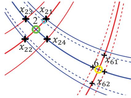
**Figure 5:** Schematic illustrating of the optimization process for nodes 2 (green) and 6 (yellow). Thin solid and dashed lines are the support trajectories, crosses refer to the design variables. The first concomitant design variable of  $x_{21}$  is  $x_{61}$ .
