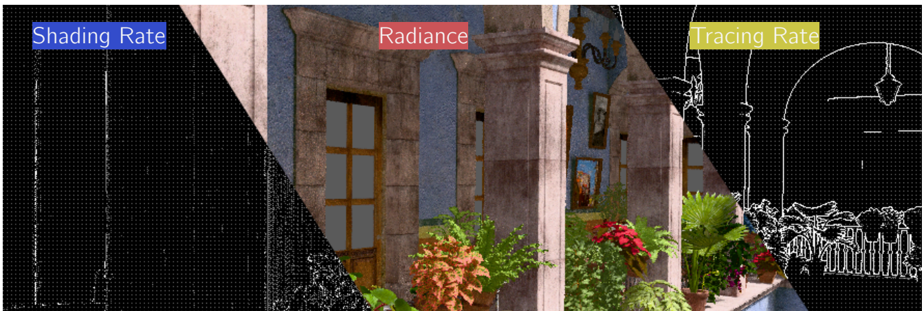
Figure 1: Our method maintains a cache of stable samples suitable for adaptive blending of the images in a stereo pair. This leads to better temporal stability and better stereo consistency. The stable samples further enable us to reduce the performance hit by using adaptive shading and adaptive visibility tracing. Shading Rate and Tracing Rate indicate the values we use to dynamically control these adaptive techniques.
