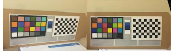
Fig. 1. Registration results. Left image is taken at an angle; the bottom has been corrected for projection. All of the images are registered, so they can be aligned and overlaid to compare targets.
