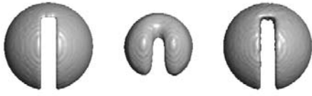
Figure 6: 360° rotation of Zalesak's sphere (100 advect-ions): initial, LS, and PLS. 524,288 particles, 128 3 grid, 14.74 FPS.
