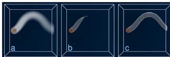
Figure 1: Dye advection of a spherical volume in a time-dependent sine wave. The injection volume is marked in red. The flow spreads the dye over time and the resulting trace depends on the computation of this process. Diffusive advection (a), level set advection (b), PLS advection (c) – ( 64^3 grid, 262,144 particles, rendering speed: 78.2, 55.9, 36.6 FPS).
