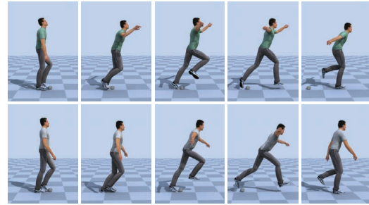
Figure 9: Results of simulating a lowering strategy with a flight phase. Top: motion capture data, and bottom: simulated result. From left to right: Passive Reaction, Clearance, Flight, and Single Support After Step.
