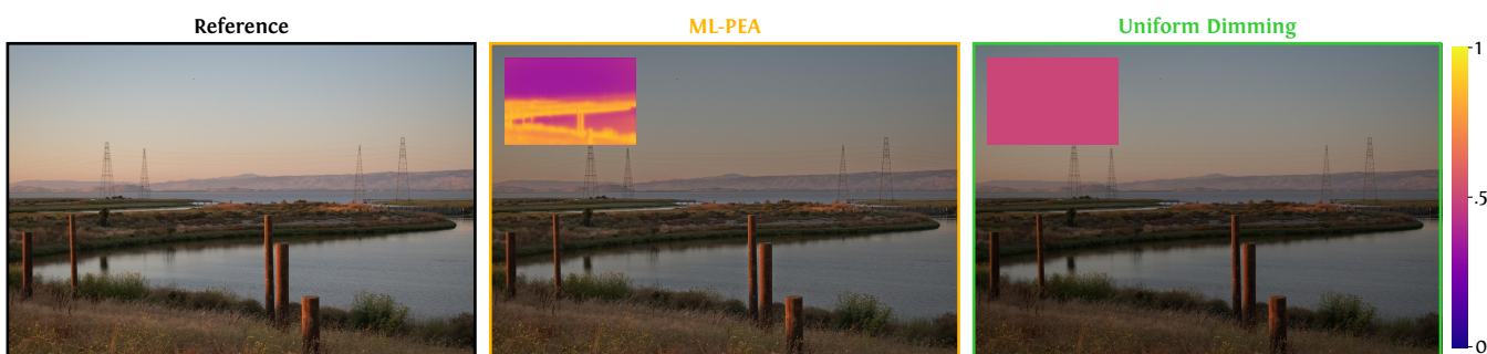
Figure 1: Our pipeline generates images which consume less power than the original when shown on a display, while minimizing perceptual impact. Here, we show an example of an image generated with our technique (●) compared to the reference (●) and its uniformly dimmed version (●). The corresponding dimming maps are shown in the insets, with the multiplicative scaling factor presented in the color bar on the right. Note that both the uniformly dimmed image and the image generated with our technique in this figure consume the same amount of display power: 52.1% of the reference.
