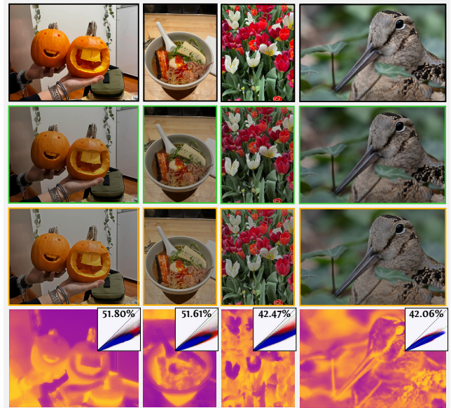
Figure 5: Example input images outside of the training dataset are shown here. We show the reference (●), uniform dimming (●), and ML-PEA (●) images as well as the dimming maps (see Figure 1 for scale). Plots of the mapping (similar to Figure 4) between reference and ML-PEA outputs are shown in the top right of each dimming map. Matched power savings are shown in the inset plots.
