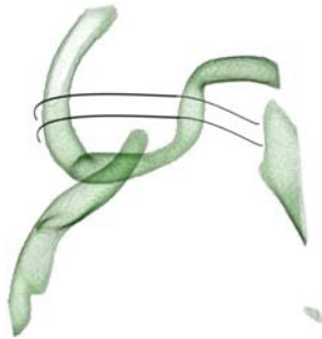
Figure 2: The image depicts change over time in a feature for CFD data. The rightward motion of the flow feature is conveyed using speedlines.
