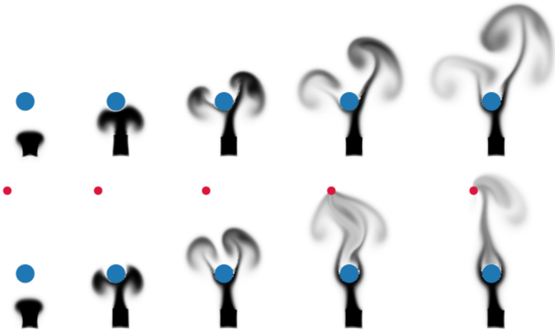
Figure 5.16: Buoyancy and divergence control (resolution 256^2 ). We simulate a hot smoke plume rising toward a blue circular obstacle in 2D using the Boussinesq buoyancy model (left). We can also add a velocity sink to the scene, indicated with a red dot, causing the smoke to be sucked into the sink (right).
