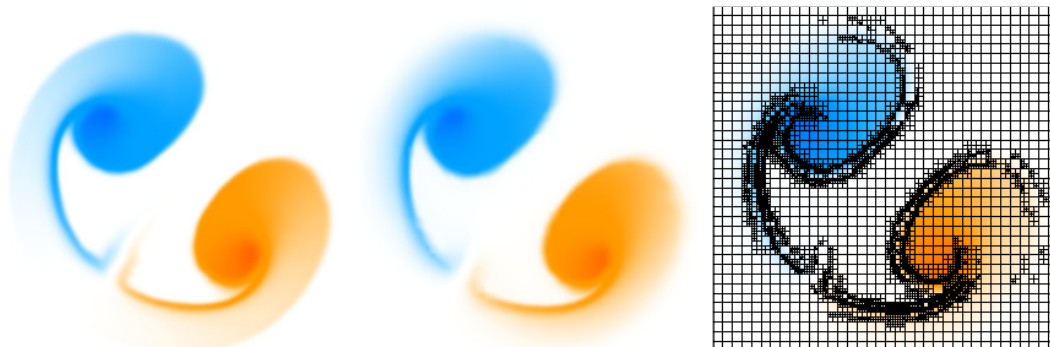
Figure 5.20: Fluid simulation results using a uniform cache (left) and an adaptive cache (middle) using one-twentieth memory footprint that of the uniform one. Slowly varying regions are sparsely cached while dense sampling occurs in regions exhibiting steep or discontinuous variations.
