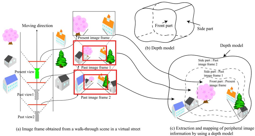
**Figure 1:** Extraction of peripheral image information by using an approximating depth model
