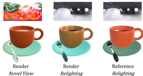
Figure 1: Challenges of relighting: After material and light estimation, (left) rendering novel view in estimated light looks reasonable. However, (middle) erroneous disentanglement of light and material degrades the reconstruction when relighted. (right) Reference. Used renderer: NvDiffRec [MHS*22].
