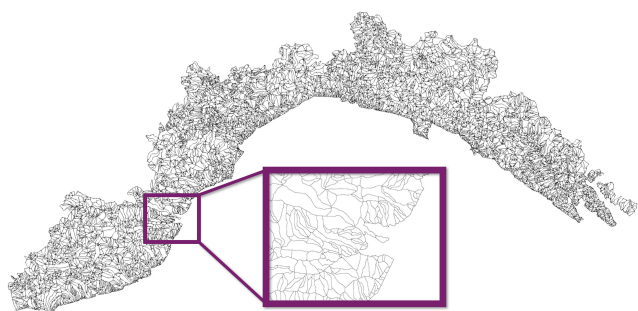
Figure 8: Example of a polygonal mesh obtained by processing a vector standard file, composed of a series of polygons representing units with homogeneous geological properties.
