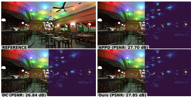
Figure 4: Comparison of our method with the NPPD and DC baselines on the Bistro3 [Lum17] scene at 8 spp. Our approach (w/pyramid) reduces errors around the light source by leveraging path-tracing inputs. Unlike DC, which tends to introduce artifacts under low-spp conditions, our generalized fusion of multiple correlated inputs effectively suppresses such artifacts.
