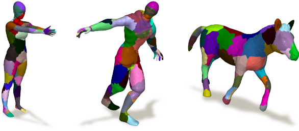
Figure 2: Illustrations of patches which tile the surface of respective 3D shapes. All patches together cover the whole surface of the shape and each individual patch has a single boundary. See Section 5.1 on how we extract patches.
