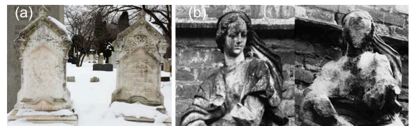
Figure 3: Photographs of stone weathering. (a) shows two similar tombstones at different weathering stages. (b) shows a stone statue before and after years of weathering. Figure (b) is reproduced from Fig. 1 in [Win87], © Springer-Verlag NY 1987. Included here by permission.
