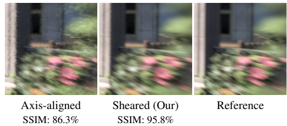
Figure 9: SAN MIGUEL 1 at 4 spp, reconstructed using an axis-aligned filter vs. our sheared filter.
