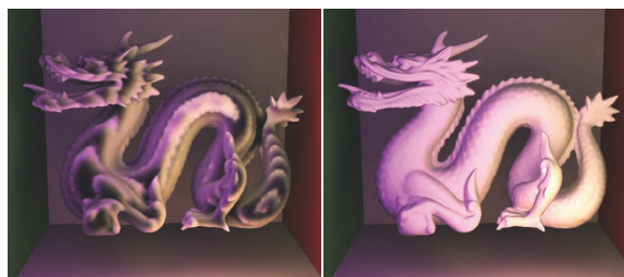
Figure 12: A dragon with self-occlusion artifacts due to limited voxel resolution. A bias helps alleviate the problem.
