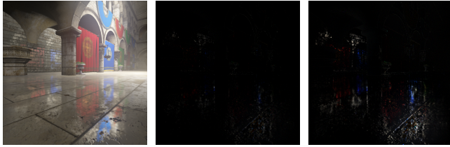
Figure 7: By terminating long rays, a performance versus quality trade is achieved. The above images show the ground truth with no terminated rays (6ms, left), the difference, multiplied by 8, to terminating up to 1 ray per warp (5.4ms, middle) and up to 4 rays per warp (4.7ms, right).
