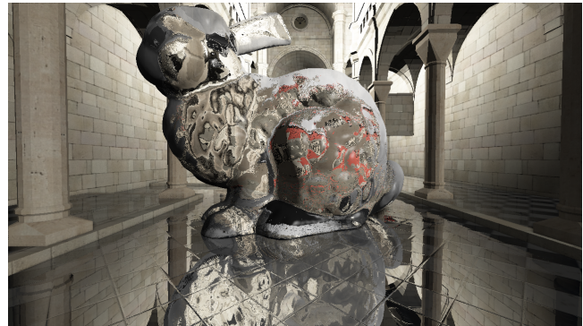
Figure 17: Refraction and reflection: The floor reflects rays that refract (twice) through the bunny (trace time 11.5 ms).
