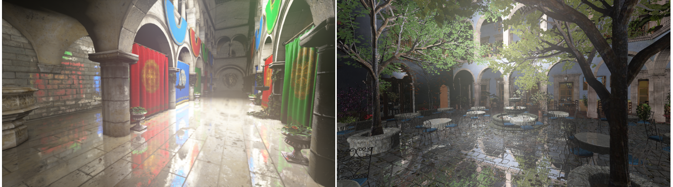
Figure 1: With our hierarchical multi-layer ray tracer, advanced effects, especially from long rays, can be rendered efficiently. Both images shown demonstrate two-bounce screen-space reflections. Note the reflection of the red and blue curtains in the left-most part in Sponza and the reflections in the windows of San Miguel. Render times for multi-layer framebuffer generation are 1.34 ms, computing our hierarchy takes 1.98 ms and tracing two reflections bounces 4.93 ms (left), and render 5.62 ms, hierarchy 2.09 ms and tracing two bounces 5.25 ms (right). All at 720p with 4 layers on Geforce 1070 GTX without any further common optimizations such as sub-sampling or increased strides.
