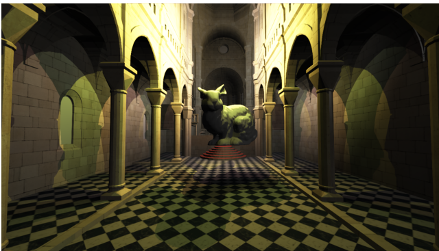
Figure 19: Shadows from 3 point lights traced by screen-space ray marching at 10.1 ms (HSSR) and 24.4 ms (SSR).
