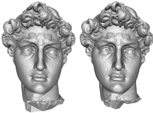
Figure 2: Surface reconstruction using Haar wavelets (left) results in a noisy surface because the basis functions are discontinuous. Smoothing the indicator function results in a substantially smoother surface at a small cost to speed and approximation quality (right).
