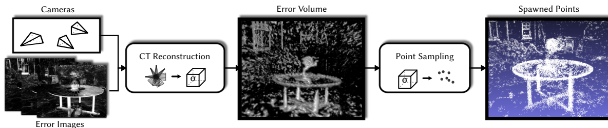
Figure 3.3: Visual Error Tomography: starting from error images ( left ), we apply computed tomography to reconstruct a 3D error volume grid ( center ). Within each voxels, random points are spawned, where the number of spawned points depends on the voxel’s error value ( right ).
