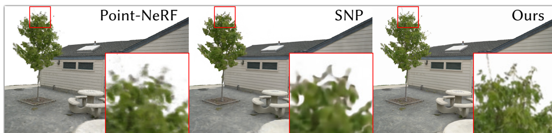
Figure 3.10: Point-NeRF [Xu et al. 2022b] and SNP [Zuo and Deng 2023] use different point spawning strategies with growing and error projection. Both fail to reconstruct fine details.
