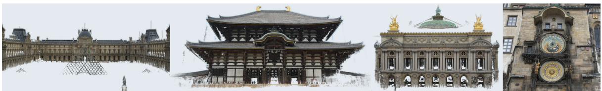
Figure 2.3: Examples of COLMAP’s dense reconstruction [Schönberger et al. 2016]. Promising results can be seen, but holes and artifacts are still visible in the point clouds. The figure is taken from the COLMAP project page [Schönberger 2024] based on Schönberger et al. [2016]. Reprinted with permission from Springer Nature Customer Service Centre GmbH: Springer Nature, ECCV, ©2016.
