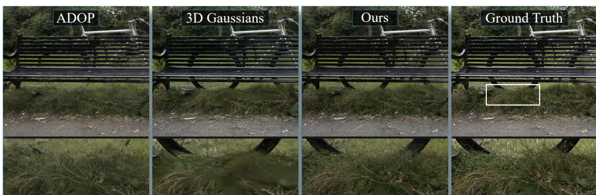
Figure 4.1: Previous point-based radiance field rendering methods provide great results in many cases, but renderings can be aliased and incomplete (ADOP [Rückert et al. 2022] (left), missing parts of the bike’s tire), or overblurred (3DGS [Kerbl et al. 2023] (middle), missing fine grass details). Our approach combines the advantages of both to render crisp, complete, and alias-free images.
