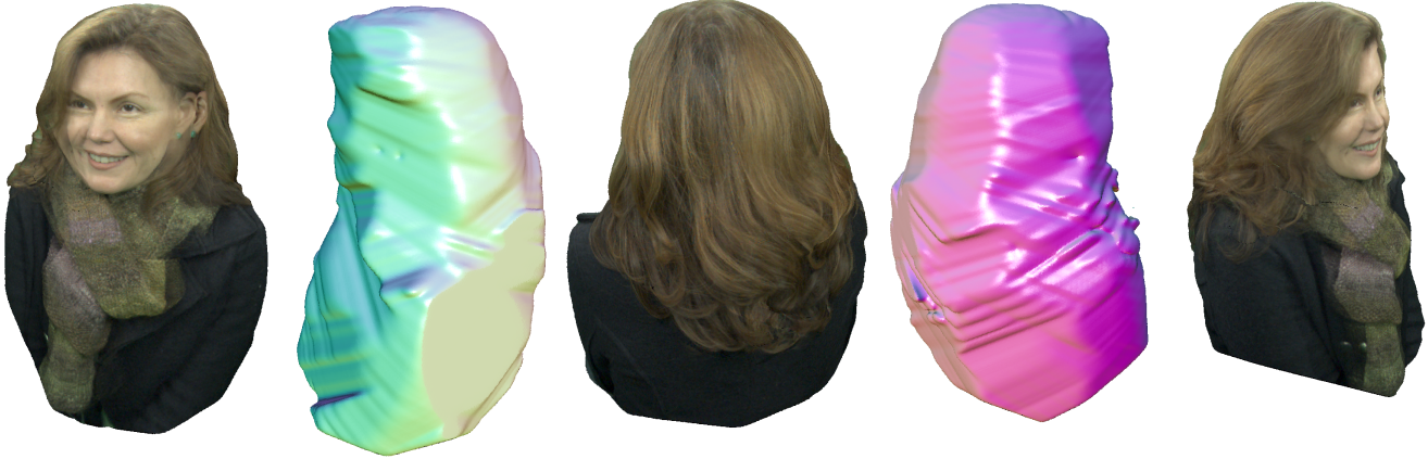
Figure 1: Several views of a model, with and without texture, reconstructed from eight cameras. This surface contains 2.5 million out of 1024^3 voxels. Computation plus rendering took 24 milliseconds.
