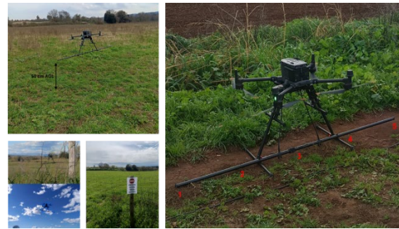
Figure 1. R4 MagDrone system testing. Possibility of access to cultivated or private lands. On the right, representation of the arrangement of the five sensors inside the horizontal magnetic bar, placed below the drone.
