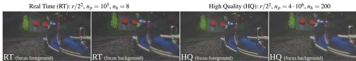
Figure 1: We introduce a fast rendering framework for Point-Based Computer Generated Holography. Our system is capable of generating visually pleasing holograms in real time (left), while adaptively changing the amount of points for better quality results (right), providing a flexible way of finding the right balance. Furthermore, our method accounts for visibility changes due to parallax and depth of field.
