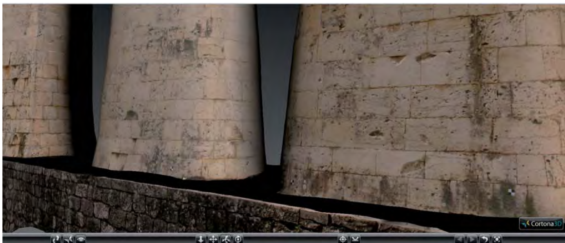
Figure 9: Detail of the final 3D textured model captured through the Cortona 3D viewer in order to give an example for the quality and resolution of the textured maps created by the proposed methods
