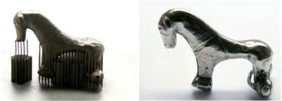
Figure 12: Fibula, Celtic. Selective Laser Melting (SLM). Source: RP-Lab, Aachen University of Applied Sciences, Celtic Museum, Hallein, Austria
