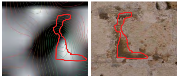
Figure 14: Visual comparison of the laser intensity and close range photographs
