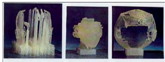
Figure 4: Bust of queen Tiye. Main elements made by AM. Scale: 2:1. Stereolithography. Source: CP-GmbH
