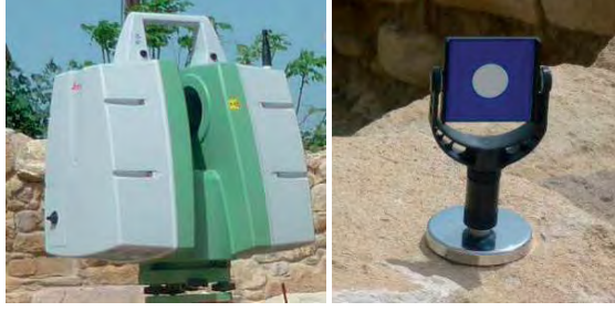
Figure 7: Leica ScanStation C10 (left) and the special targets (right)
