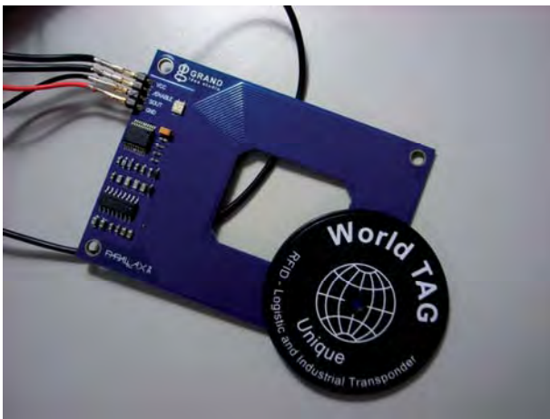
Figure 4: RFID reader and Tags
