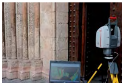
Figure 2: HDS ScanStation 2 during the data acquisition
