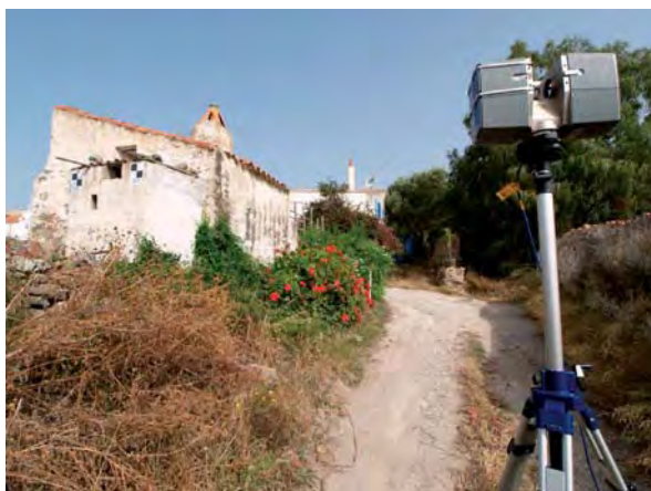
Figure 6: The laserscan at work in the “Le Tanche” settlement
