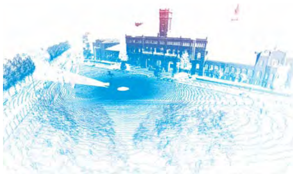
Figure 10: Terrestrial laserscan with color indicating height
