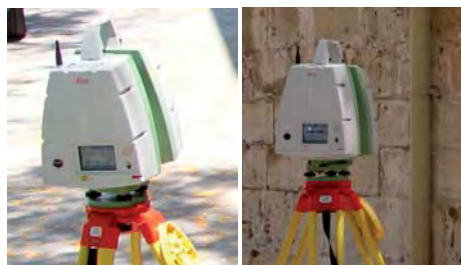
Figure 5: The Laser ScanStation C10 used
