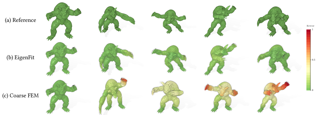
Figure 1: Numerical stiffening can cause animations on a coarser FEM mesh (sequence (c)) to deviate from corresponding ones on a finer mesh (sequence (a)). To fix this error, EigenFit adjusts the magnitudes of the leading modes on the coarse mesh using the fine mesh at rest state, resulting in sequence (b). The meshes are coloured by normalized positional error with respect to the finer mesh. EigenFit often outperforms current leading alternatives.
