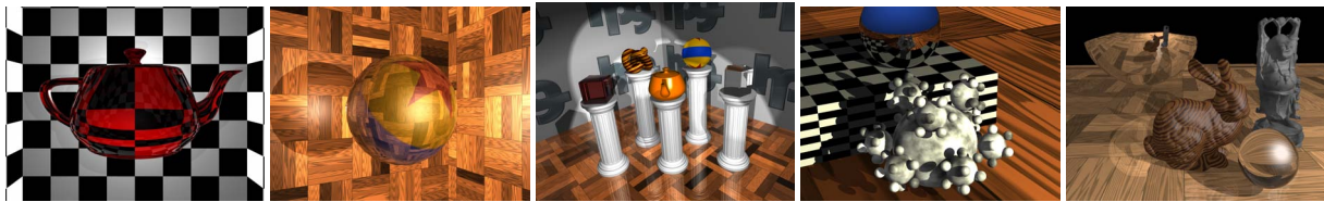
Figure 3: Scenes rendered with RTfact, Manta (2nd from right), and PBRT (rightmost). The surface shaders are written in RenderMan or scalar C++ and all compiled to a platform-independent intermediate representation. The AnySL system loads, vectorizes, and optimizes the shaders and seamlessly integrates them into the renderer at runtime, achieving close to native shading performance.
