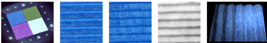
Figure 3.21: From left to right: Unprocessed HDR image from the raw dataset, extracted and rectified texture for an orthogonal view ), extracted and rectified texture for a grazing view , reconstructed height field, BTF rendering with parallax mapping under point light illumination.
