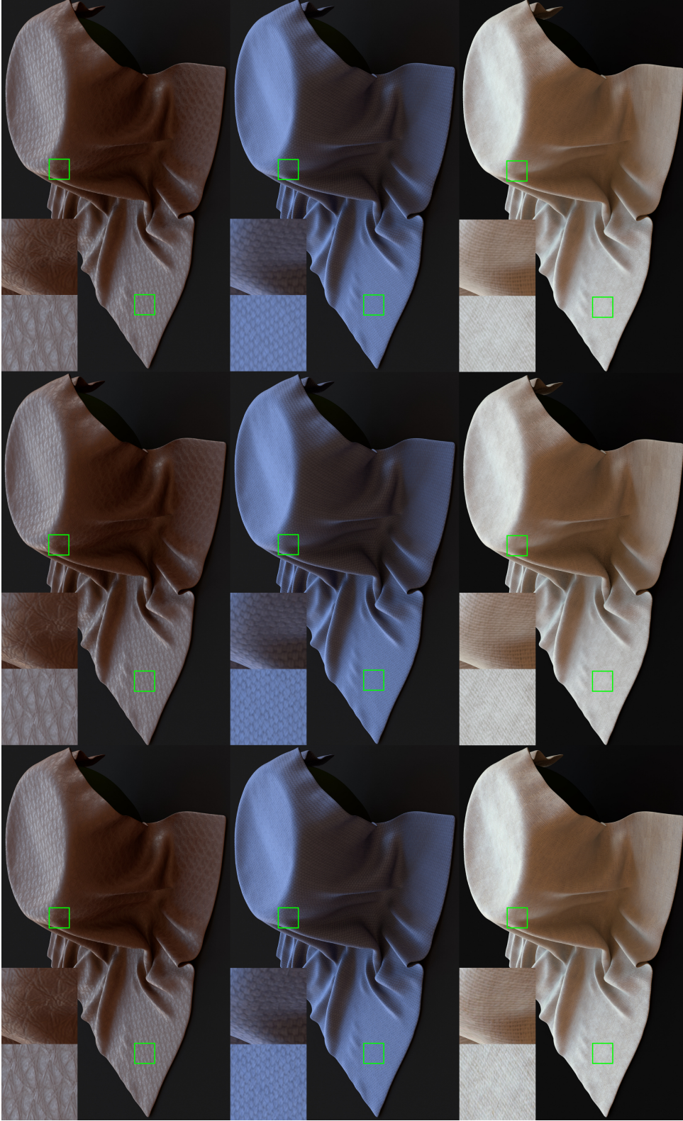
Figure 4.12: Renderings with Mitsuba's pathtracer ( 2000 \times 1200 pixels, 128 samples per pixel, 10 processes, uniformly sampled BSDFs, environment lighting). Left to right: original BTTF, our network and PCA. Datasets (left to right): leather04, fabric04, cotton.
