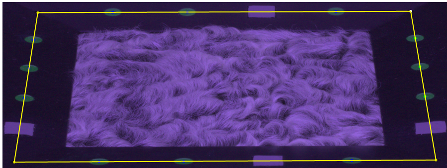
Figure 3.10: Detection of the sample holder frame (highlighted in yellow) in a photograph under diffuse modeling light (which causes the purple tint).
