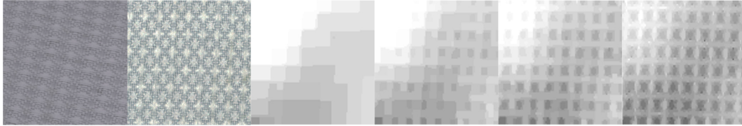
Figure 3.13: Left to right: Close-up view of the material from a grazing angle under diffuse ceiling light, one extracted BTf texture and different reconstructed height maps for decreasing smoothness coefficients (0.002, 0.0002, 0.0001, 0.00002). All scalar height maps are gamma-corrected for display. Dataset: whi temesh from our database.
