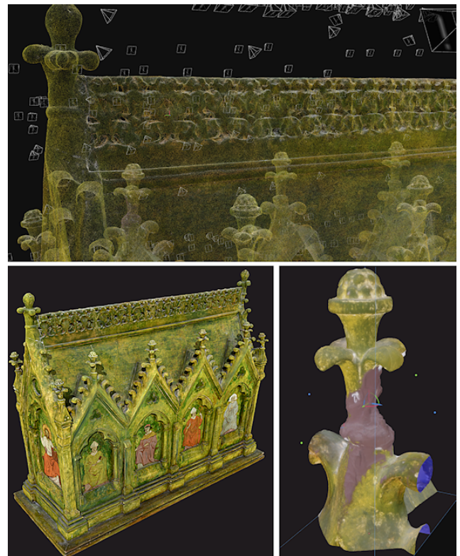
Figure 1: Reconstruction of the shrine of St Livinus (Sint-Lievens-Houtem, Church of St Michael), Sketchfab rendering (200.1k triangles simplified model) for public presentation of the collection, and the 3D detail of a problematic restoration.
