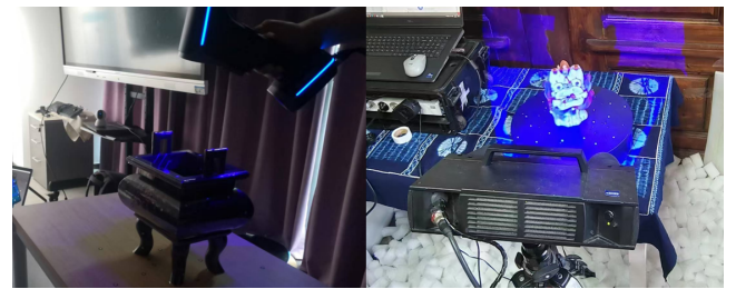
Figure 3: we use the 3D scanners to obtain the ground truth mesh.
