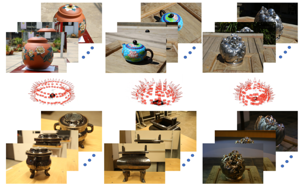
Figure 2: We collect data along the loop of the upper hemisphere, and use the COLMAP [SF16] to obtain the camera's intrinsic and extrinsic parameters.
