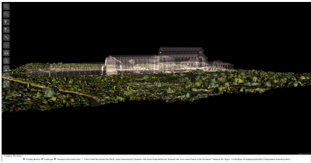
Figure 10: Data hosted in 3DHOP, with the visualisation of 3 layers and other tools for interacting with the 3D model.
