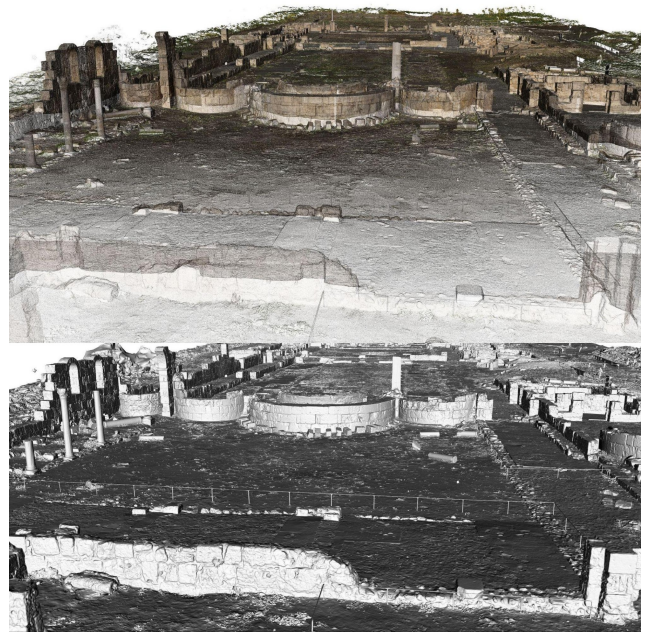
Figure 4: Visualisation of the 3D representation of the Basilica: high resolution 3D point cloud (upper image); high resolution mesh (lower image).
