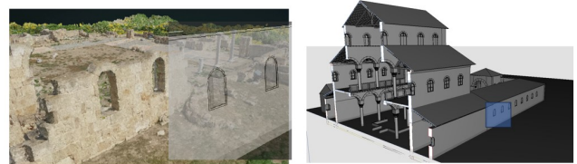
Figure 6: Shape extraction from the 3D Model of the existing condition.
