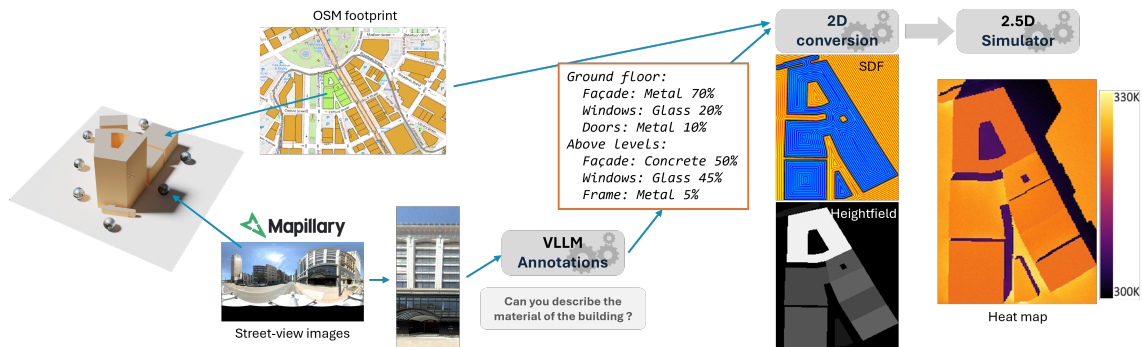
Figure 1: We propose a pipeline for estimating the facade composition of buildings in a city, linking this information with their thermal properties to feed our 2.5D heat transfer simulator. First, we combine OpenStreetMap data with geolocated street-view 360° images to identify the best image for each building, which we input into a VLM to query the facade composition. We represent the city fully, including its materials and geometry, in randomly accessible 2D maps, which serve as inputs for our simulator that models coupled heat transfers.
