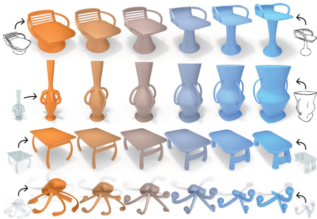
Figure 16: Shape interpolation. We uniformly interpolate between two (left and right) GeoCode shapes. Interpolations contain gradual changes (continuous parameters) as well as sharp structural changes (discrete or binary parameters).
