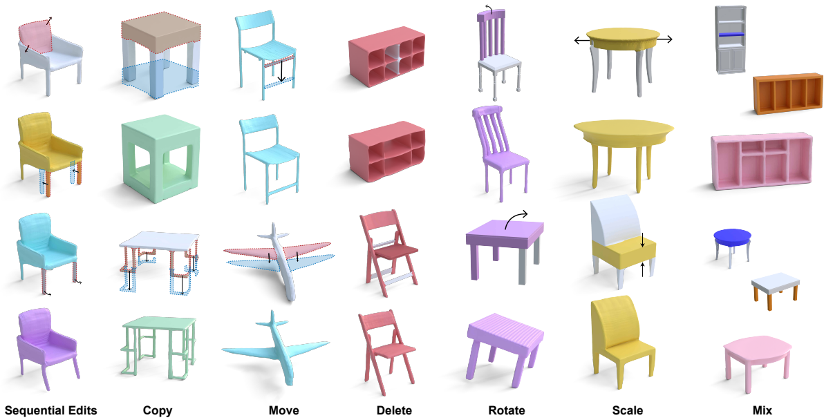
Figure 1: Part-level editing results produced by SPLICE . Our method supports a wide range of intuitive editing operations, including sequential edits, copy, move, delete, rotate, scale, and mix, without requiring manual post-adjustment. The edited shapes remain structurally coherent and visually plausible. Additionally, SPLICE exhibits strong robustness under multi-step editing, consistently maintaining high reconstruction quality throughout the editing process.
