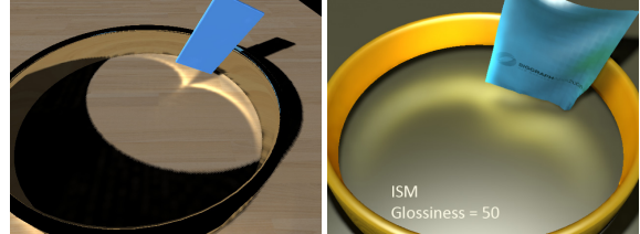
(c) Ours Support high-freq reflection. 60Hz on Geforce 260 GTX (d) ISM [RGK*08] Only slightly glossy. 13Hz on Geforce 8800 GTX
